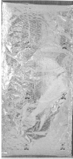
(a) Glass Wool with foil face up and PVC sheet facing down
